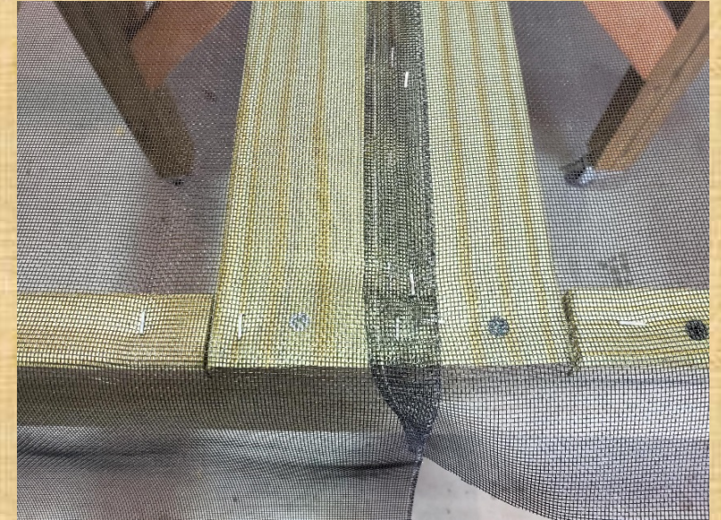
Stapled screen- 2 pcs- attached in the middle- 6ft each
