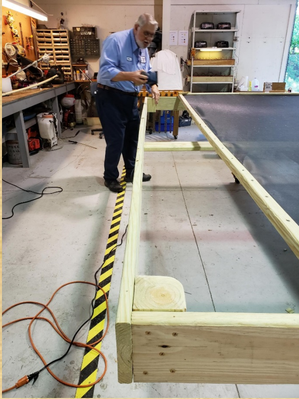
Screen top made with 1x2 plywood
