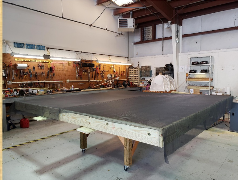
Top frame attached to bottom frame for stability while attaching screen and 2 nd 1X2.
